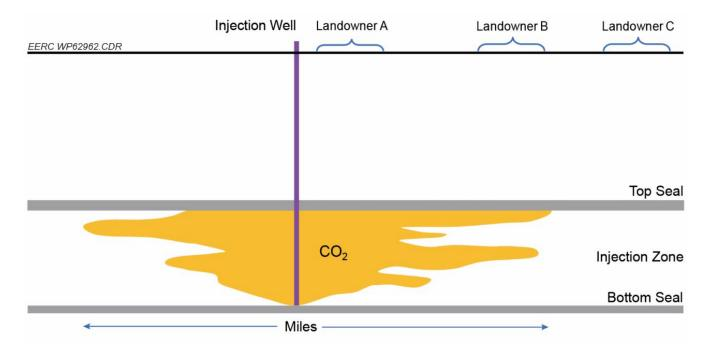
Figure 4. Cross-sectional view depicting a CO<sub>2</sub> plume in the subsurface.
